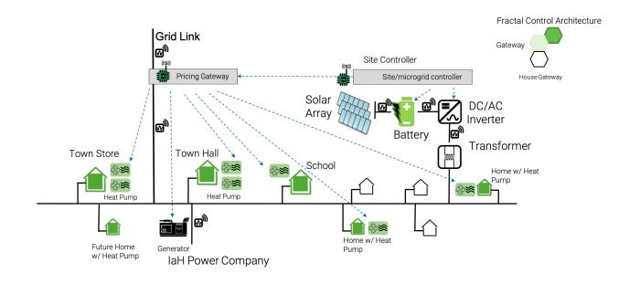
The IaH microgrid uses real-time pricing signals and controls to turn heating loads into flexible (active) demand resources that **respond to changes in the abundance or scarcity of power**. This integrated solution uses Air to Water heat pumps with thermal storage and machine learning algorithms allowing the heat
